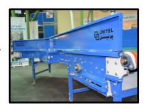
The drive pulley is driven by integral reducers, either shaft mounted or sprocket driven. The drive unit could be also of the center-drive type with its integral belt tensioning system.
