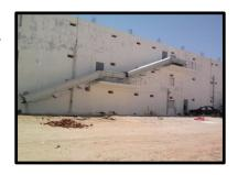
HYB conveyors can be floor mounted, suspended from ceilings using hangers, or wall mounted using brackets
